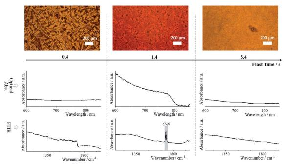
Fig. 1 Film evolution during annealing. Optical images are measured in transmission mode. Optical absorption spectra, and FTIR measurement were performed on a single spot for FA<sub>0.85</sub>MA<sub>0.1</sub>Cs<sub>0.05</sub>PbI<sub>3</sub> perovskite composition and three flash times.
