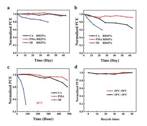
Fig. 5 Stability measurements: (a) at room temperature with humidity  $25\pm5\%$ , (b) at room temperature with humidity of  $45\pm5\%$ , (c) at  $85\,^{\circ}\text{C}$  in an N<sub>2</sub>-filled glovebox for the 3D and 2D PVSCs. (d) Thermal-cycling test for the PMA-based device.
