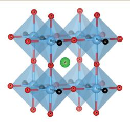
Fig. 1 The crystal structure of the ABX<sub>2</sub>Y perovskite used for the highthroughput search. The orange ball denotes the A atom, while cyan balls are B atoms, green balls X atoms and pink balls Y atoms. The unit cell is tetragonal with space group P4/m2/m2/m (#123). Image produced with VESTA.40
