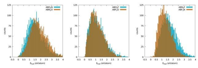
Fig. 2 Distribution of the distances to the convex hull of all oxynitride (left), oxyfluoride (center), and nitrofluoride (right) perovskites. The bins have a size of 40 meV per atom.
