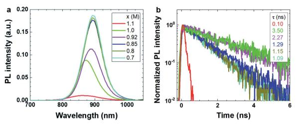
Fig. 4 PL measurements of  $PEA_{0.08}FA_xSnI_3$  films. (a) Steady state and (b) time-resolved PL. The color scheme is the same in the two figures, lifetimes are reported in the legend of (b).
