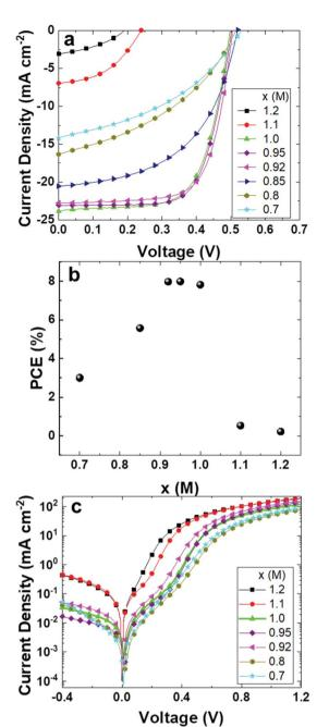
Fig. 6  $PEA_{0.08}FA_xSnI_3$  based devices. (a) J-V curves under AM 1.5G conditions, (b) PCE versus FA concentration and (c) J-V curves of the solar cells under dark conditions. Displayed results are coming from a batch of consistent samples.
