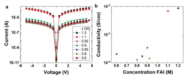
Fig. 5 Conductivity measurements of PEA<sub>0.08</sub>FA<sub>(x)</sub>SnI<sub>3</sub> films. (a) I-V characteristics under dark conditions, and (b) electrical conductivity calculated from the I-V curves in (a).
