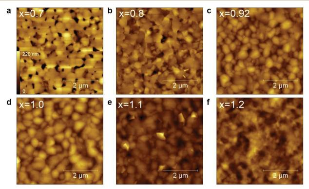
Fig. 3 AFM images of PEA $_{0.08}$ FA $_x$ SnI $_3$  at a scan area of 5  $\mu$ m  $\times$  5  $\mu$ m.
