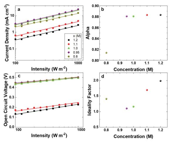
Fig. 7 (a)  $J_{SC}$  as a function of the light intensity, (b) the extracted values of  $\alpha$ , (c)  $V_{OC}$  as a function of the light intensity and (d) the extracted ideality factor n for the solar cells.
