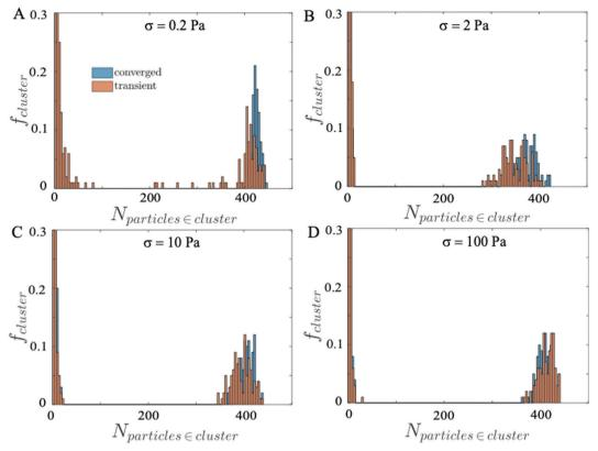
Fig. 9 Simulation results of the average size distribution of particle clusters at different shear stress values ( $\sigma$  = (A) 0.2 Pa, (B) 2 Pa, (C) 10 Pa, (D) 100 Pa) for strongly attractive suspension of  $\alpha = 0.4$  M and  $\phi = 0.46$ . Orange and blue bars represent the transient and converged states, respectively. The total number of particles in the simulation is 512
