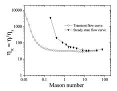
Fig. 6 Relative viscosity ( $\eta_R$ ) versus the Mason number (Mn) at  $\phi=0.46$  and  $\alpha=0.4$  M from the flow curve measurements. Open circles represent the data obtained from the transient flow curve with the waiting time 450 s while the filled triangles represent the steady flow curve obtained with the waiting time 2000 s.
