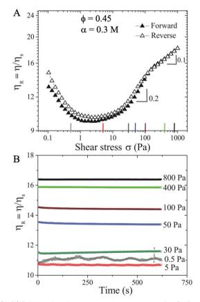
Fig. 2 (A) Relative viscosity  $\eta_R$  versus shear stress  $\sigma$  at  $\phi=0.45$  and  $\alpha=0.3$  M. Forward and reverse flow measurements correspond to filled and open symbols, respectively. (B) Temporal behavior of  $\eta_R$  for an applied  $\sigma$ . The colored vertical lines in (A) correspond to the  $\sigma$  values in (B).
