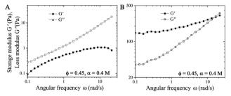
Fig. 5 Storage modulus (G') and loss modulus (G'') versus the angular frequency ( $\omega$ ) from the frequency sweep measurements performed (A) immediately after the forward flow curve measurements where  $\sigma$  is increased from 0.1 to 1000 Pa, (B) after shearing the suspension at  $\sigma_y$  = 1 Pa. The strain amplitude is fixed at 1%.
