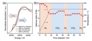
Fig. 5 (a) In situ Mo K-edge XANES spectra of Pt/MoO $_3$  measured at 200 °C; before H $_2$  reduction (black line), after H $_2$  reduction under a flow of 20% H $_2$ /He (red line), after subsequent flow of 20% CO $_2$ /He (blue line) and subsequent flow of 20% H $_2$ /He (orange line). (b) Change of valence state of the Mo species during the in situ XAFS measurement. The valence state was determined by a linear interpolation method
