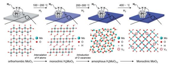
Scheme 1 Schematic illustration of the crystallographic changes of  $Pt/H_xMoO_{3-v}$  upon  $H_2$  reduction.
