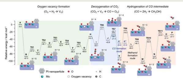
Fig. 8 Optimized reaction pathway for  $CO_2$  hydrogenation to produce methanol, and potential energy diagram obtained by DFT calculation using  $H_{26}Mo_{32}O_{96}-Pt_{20}$  slab model and schematic illustrations of the corresponding structure models in each reaction step.
