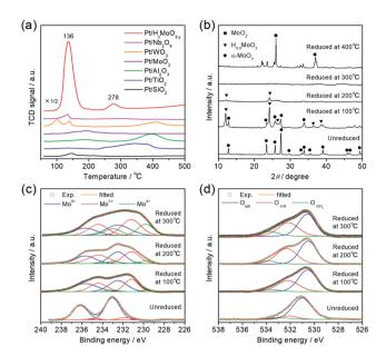
Fig. 3 (a)  $H_2$ -TPR profiles of Pt catalysts supported on various metal oxides. (b) XRD patterns, (c) Mo 3d XPS spectra, and (d) O 1s XPS spectra of unreduced Pt/MoO<sub>3</sub> and Pt/H<sub>x</sub>MoO<sub>3-y</sub> catalysts reduced with  $H_2$  at different temperatures.
