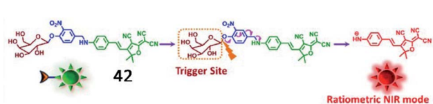
Fig. 32 Conceptual scheme of 42 when encountering \beta -galactosidase. Reprinted from ref. 129 with permission. Copyright 2017 Elsevier Ltd.
