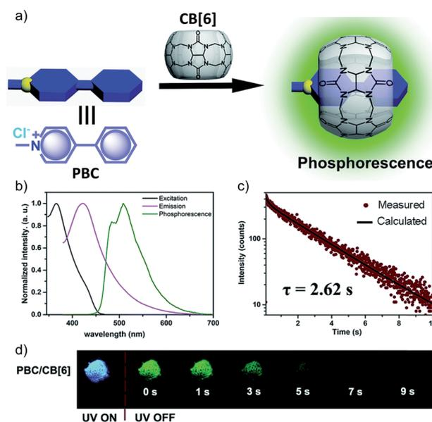
Fig. 7 (a) Schematic illustration of the solid-state supramolecular strategy of PBC and **CB[6]** for URTP. (b) Excitation, emission, and phosphorescence spectra of **PBC/CB[6]** in the solid state. (c) Phosphorescence decay of **PBC/CB[6]** at 510 nm. (d) Photographs of **PBC/CB[6]** powder under 365 nm UV irradiation and at different time intervals after removal of the ultraviolet lamp. Reproduced with permission from ref. 96. Copyright 2019, Royal Society of Chemistry.
