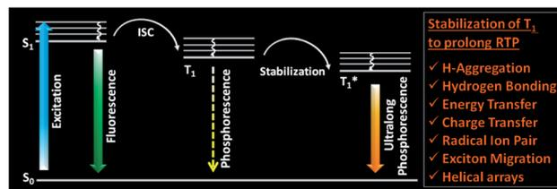
Fig. 1 Schematic of stabilization of the triplet state, leading to ultra-long phosphorescence in organic molecules.
