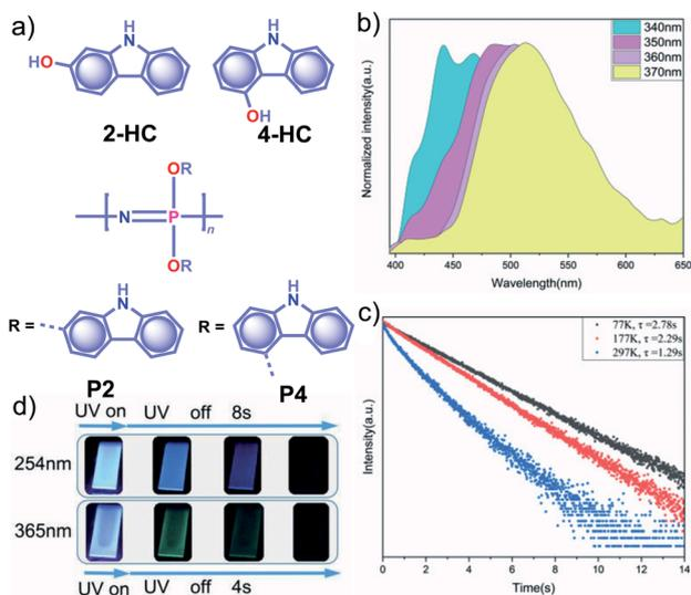
Fig. 10 (a) Chemical structure of monomers **2-HC** and **4-HC**, and polymers **P2** and **P4**. (b) Excitation wavelength-dependent phosphorescence spectra and (c) temperature-dependent phosphorescence decay curves of **PVA-100-P4-1** film. (d) Photographs of persistent luminescence of **PVA-100-P4-1** film under ambient conditions. Reproduced with permission from ref. 112. Copyright 2020, WILEY-VCH.
