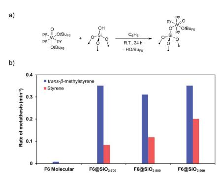
Fig. 6 (a) Preparation of well-defined silica-supported W(w) oxo species. (b) Rates of metathesis of trans- $\beta$ -methylstyrene (blue) and styrene (red) catalysed by W(w) oxo species, molecular and supported on silica prepared at different dehydroxylation temperatures. Reprinted with permission from ref. 164. Copyright 2019 American Chemical Society.
