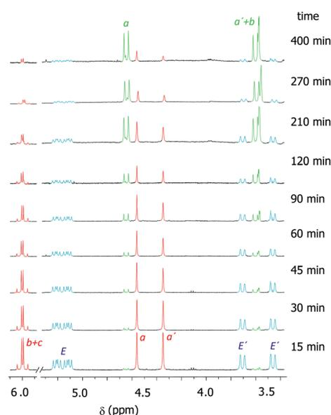
Fig. 1 Kinetic experiment of the cyclization of **1a** (DMF, 1 equiv. CsOH, 25 °C, 25 mM). Signals referred to **1a** are in red (thread) and light blue (macrocycle). Signals of the forming lactam *trans*-**2a** are in green. For lettering see Table 2. Note that the signals referred to the macrocycle (E and E') in *trans*-**2a** appeared as very broad peaks, being difficult their observation at room temperature (see ESI for further details†).
