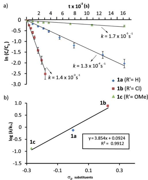
Fig. 2 Cyclization of rotaxanes **1a**–**c** in the presence of CsOH (1 equiv.) at 25 °C in DMF: (a) Plots of  $\ln(c/c_0)$  versus time for the determination of the rate constants; (b) Hammett plot of  $\log(k/k_{1a})$  against the substrate electronics ( $\sigma_p$ ). The rate constant values are the average of two independent measurements.
