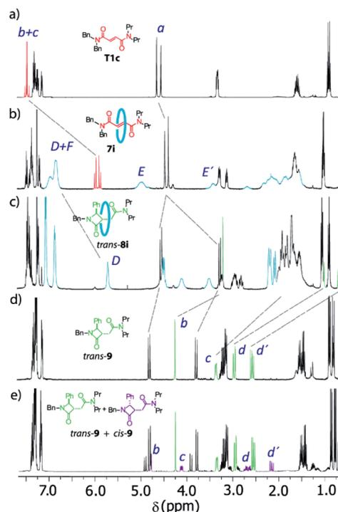
Fig. 8 <sup>1</sup>H NMR spectra (400 MHz, CDCl<sub>3</sub>, 298 K) of (a) *N,N*-dibenzyl-*N',N'*-dipropylfumaramide **T1c**; (b) fumaramide-based [2]rotaxane **7i**; (c) interlocked  $\beta$ -lactam *trans*-**8i**; (d)  $\beta$ -lactam *trans*-**9**; and (e) mixture of  $\beta$ -lactams *cis*- and *trans*-**9** obtained by cyclization of the thread **T1c**. Lettering as in Scheme 4.
