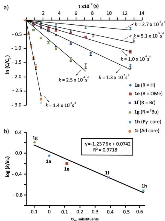
Fig. 3 Cyclization of rotaxanes **1a** and **1e**–**i** in the presence of CsOH (1 equiv.) at 25 °C in DMF: (a) Plots of  $\ln(c/c_0)$  versus time for the determination of the rate constants; (b) Hammett plot of  $\log(k/k_{1a})$  against the substrate electronics ( $\sigma_m$ ). The rate constant values are the average of two independent measurements.
