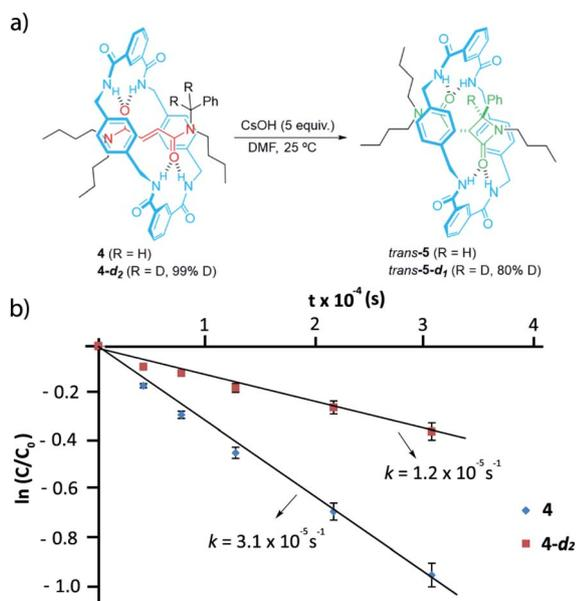
Fig. 4 (a) Synthesis of interlocked β-lactams *trans*-**5** and *trans*-**5-d<sub>1</sub>**; (b) plots of  $\ln(c/c_0)$  versus time for the determination of the rate constants of the cyclizations of rotaxanes **4** and **4-d<sub>2</sub>** in the presence of CsOH (5 equiv.) at room temperature in DMF.
