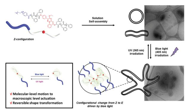
Fig. 1 Schematic representation of the reversible shape transformation of self-assembled structures of PEG-b-[OPLA] containing hydrazone-based photoswitches via configurational switching of the system.
