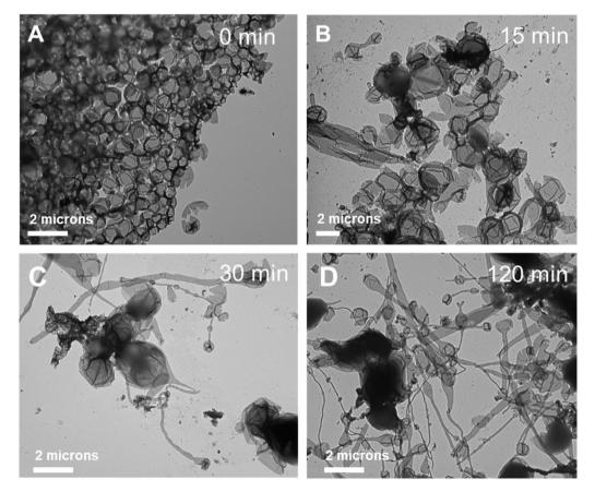
Fig. 8 TEM images of self-assembled structures of PEG1000-*b*-[OPLA<sub>4</sub>-H1-OPLA<sub>8</sub>-H1-OPLA<sub>4</sub>] under blue-light irradiation at different irradiation times. The morphologies were observed (A) before blue light irradiation and, after (B) 15 min, (C) 30 min, and (D) 120 min of blue light irradiation. The PEG1000-*b*-[OPLA<sub>4</sub>-H1-OPLA<sub>8</sub>-H1-OPLA<sub>4</sub>] samples were treated with phosphotungstic acid solution for negative staining.
