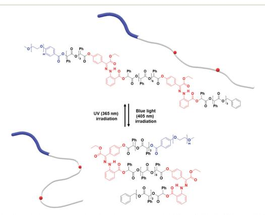
Fig. 6 Photo-induced isomerization of two photoswitches in the hydrophobic chain of PEG1000-b-[OPLA<sub>4</sub>-H1-OPLA<sub>8</sub>-H1-OPLA<sub>4</sub>].
