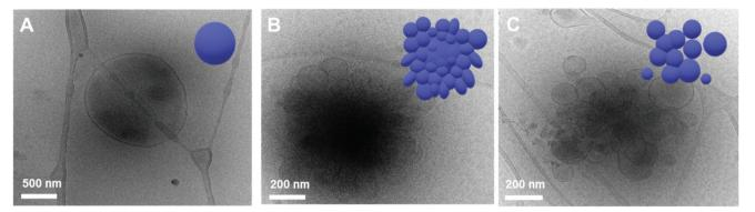
Fig. 4 Cryo-TEM images and 3D graphic representations of self-assembled structures of PEG550-b-[OPLA8-H1-OPLA9] under different light sources. The morphologies were observed (A) before and (B) after blue-light irradiation, followed by (C) UV light irradiation.
