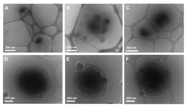
Fig. 5 Cryo-TEM images of self-assembled structures of (A-C) PEG1000-b-[OPLA<sub>8</sub>-H1-OPLA<sub>9</sub>] and (D-F) PEG1000-b-[H1-OPLA<sub>17</sub>] under different light sources. The morphologies were observed (A and D) before and (B and E) after blue light irradiation, followed by (C and F) UV light irradiation.
