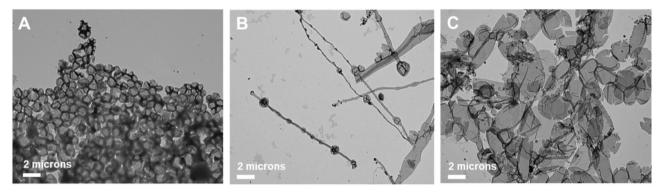
Fig. 7 TEM images of self-assembled structures of PEG1000-b-[OPLA<sub>4</sub>-H1-OPLA<sub>8</sub>-H1-OPLA<sub>4</sub>] under different light sources. The morphologies were observed (A) before and (B) after blue-light irradiation, followed by (C) UV light irradiation. The PEG1000-b-[OPLA<sub>4</sub>-H1-OPLA<sub>8</sub>-H1-OPLA<sub>4</sub>] samples were treated with phosphotungstic acid solution for negative staining.
