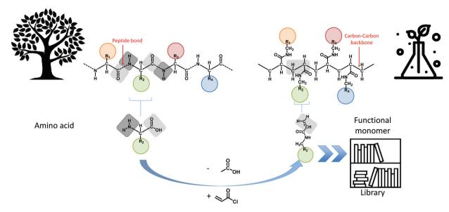
Fig. 1 Overview of the main concept of translating amino acid structures into acrylamides. A comparison between the structure of a peptide sequence and a synthetic oligomer sequence is made.
