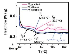
Fig. 6 (A) Differential scanning calorimetry (DSC), (B) thermogravimetric analysis (TGA) thermograms for the sequence-controlled copolymers, P3-5.
