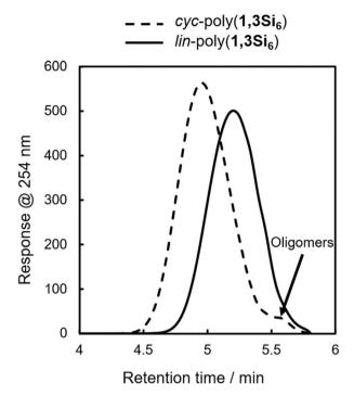
Fig. 2 GPC of cyc-poly(1,3Si<sub>6</sub>) (dotted line) and lin-poly(1,3Si<sub>6</sub>) (solid line). Determined relative to polystyrene standards at 254 nm (THF, [linpoly(1,3Si<sub>6</sub>)] = 1 mg mL<sup>-1</sup>, 40 °C, 0.35 mL min<sup>-1</sup>, 10  $\mu$ L injection).
