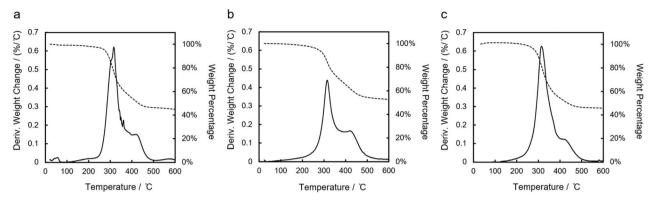
Fig. 5 TGA curves of (a) lin-poly(1,4Si<sub>6</sub>), (b) cyc-poly(1,3Si<sub>6</sub>) and (c) lin-poly(1,3Si<sub>6</sub>). Solid lines: derivative weight change; dotted lines: percentage weight change.
