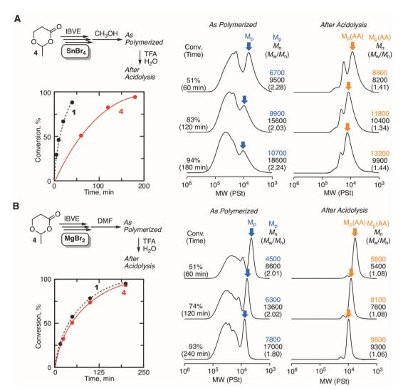
Fig. 5 Comparison between SnBr<sub>4</sub> (A) and MgBr<sub>2</sub> (B) as a catalyst for the ring-expansion cationic polymerization of IBVE with 4: [IBVE]<sub>0</sub>/[4]<sub>0</sub>/[SnBr<sub>4</sub> or  $MgBr_2|_0/[DTBMP]_0 = 380/5.0/5.0$  or 10/0.15 mM in toluene (for  $SnBr_4$ ) or toluene/ $Et_2O$  (90/10 vol%) (for  $MgBr_2$ ) at 0 °C.
