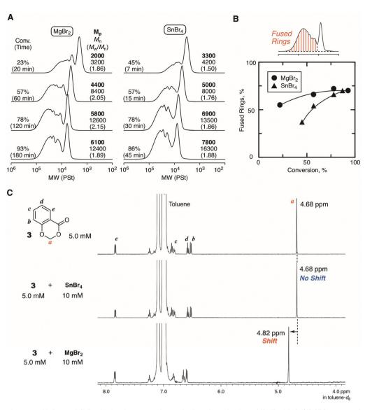
Fig. 4 Comparison between  $MgBr_2$  and  $SnBr_4$  in the ring-expansion cationic polymerization of IBVE with 1: (A) SEC curves of the obtained poly (IBVE)s (B) ratios of the fused ring estimated by peak separation. (C)  $^1H$  NMR analyses of the mixture of  $MgBr_2$  or  $SnBr_4$  with 3 as the model compound for the evaluation of the interaction with the HAE bond.
