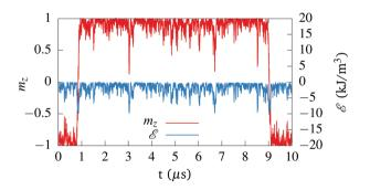
Fig. 3 Magnetisation along the anisotropy easy axis (left *y*-axis, red line) and energy density,  $\mathcal{E}$ , showing the heat extracted from and dissipated into the particle environment, as function of time. Note the two switching events around  $t=1~\mu s$  and  $t=9~\mu s$ .
