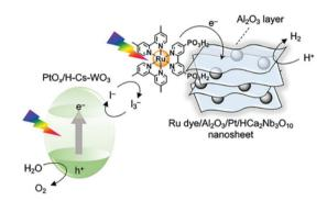
Fig. 6 Schematic illustration of Z-scheme splitting using Ru(II) trisdiimine dye for sensitization of  $Al_2O_3/Pt/HCa_2Nb_3O_{10}$  nanosheets in combination with  $PtO_x/H-Cs-WO_3$ . This figure has been reproduced from ref. 61 with permission from American Chemical Society, copyright 2020.
