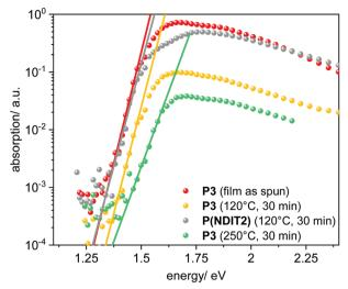
Fig. 6 Comparison between the absorption of **P3** ( $M_n = 61 \text{ kg mol}^{-1}$ ) and P(NDIT2) ( $M_n = 62 \text{ kg mol}^{-1}$ ) thin films in dependence of the annealing temperature; measured by photothermal deflection spectroscopy. The solid line displays the corresponding exponential fits for extraction of the Urbach energy  $U_E$ . Films were spin-coated (1000 rpm, 60 s) from o-DCB solutions.
