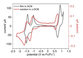
Fig. 3 Cyclic voltammograms of P(NDI-IDT) as film deposited on an ITO substrate in a 0.1 M NBu $_4$ PF $_6$  acetonitrile solution (black) and in a 0.1 M NBu $_4$ PF $_6$  o-DCB solution (red) at a scan rate of 50 mV s $^{-1}$ .
