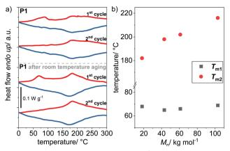
Fig. 4 (a) DSC curves of P1 ( $M_n = 18 \text{ kg mol}^{-1}$ ). First and second cycles were measured under N<sub>2</sub> with 10 K min<sup>-1</sup> before and with 20 K min<sup>-1</sup> after room temperature aging; (b) side chain  $T_{m1}$  and main chain  $T_{m2}$  melting transitions in dependence of  $M_{W}$ .
