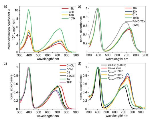
Fig. 2 Molar extinction coefficient (a) and normalized (b) UV-vis spectra of P(NDI-IDT) of different MW ( $M_n$  in g mol<sup>-1</sup>) in chloroform solution at room temperature. Solvent dependent (c) and film (d) UV-vis spectra of **P3** ( $M_n = 61 \text{ kg mol}^{-1}$ ).
