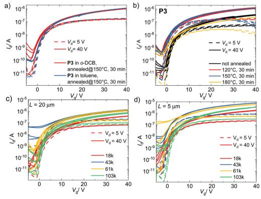
Fig. 5 Optimization of OFET devices. Effect of solvent for spin coating (a) and annealing temperature for P3 (b). Transfer curves of optimized devices as a function of MW (g mol<sup>-1</sup>) and channel length (c and d).
