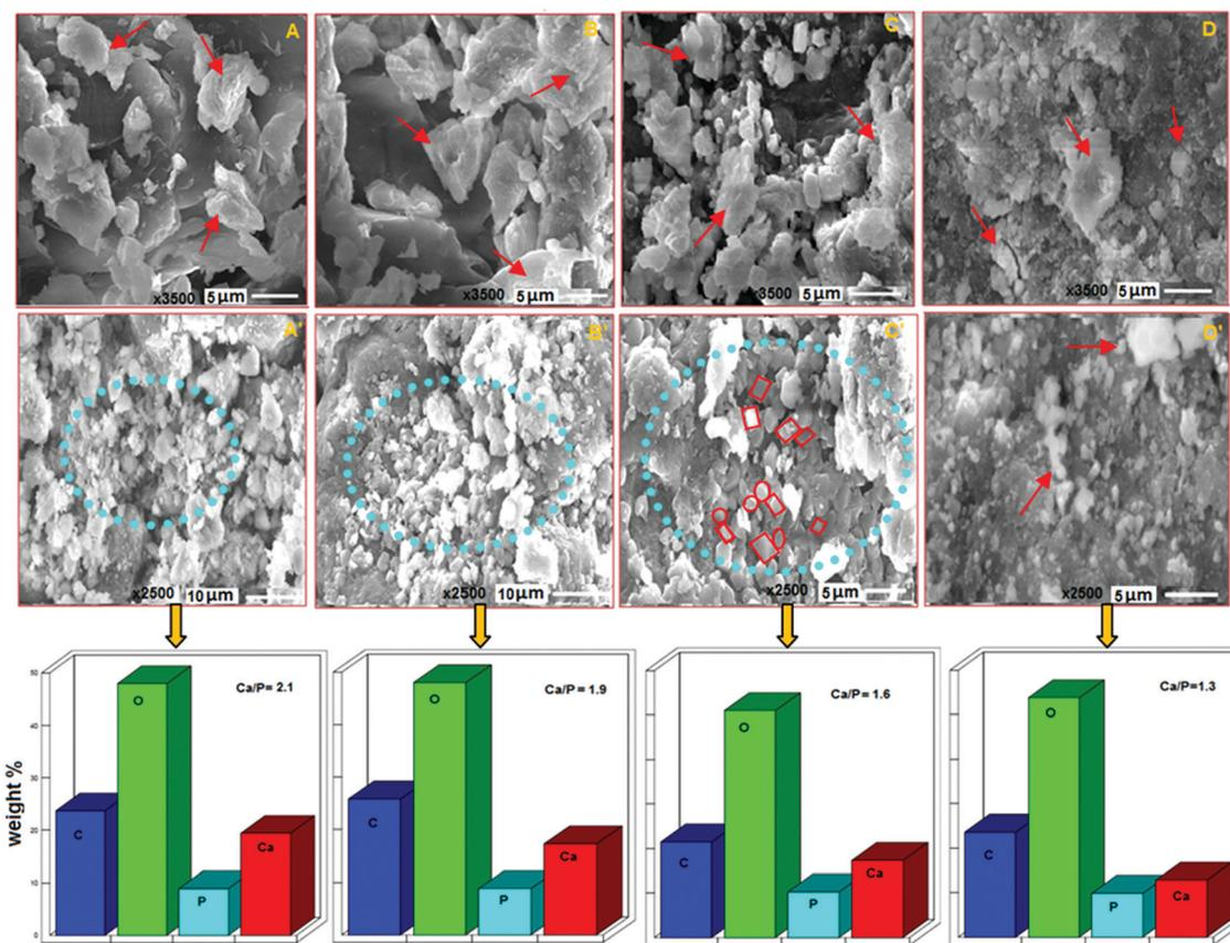
Fig. 3 Characteristic SEM micrographs illustrating the bioactivity profile by the SBF study of [A] BCHD1, [B] BCHD2, [C] BCHD3, and [D] CH nanocomposite scaffolds at 4 weeks [magnification:  $\times 3500$ , scale bar:  $5\ \mu\text{m}$ ] and at 8 weeks [A'–D'] [magnification:  $\times 2500$ , scale bar:  $10\ \mu\text{m}$ ], respectively, with their respective EDX micrographs recorded after 8 weeks.
