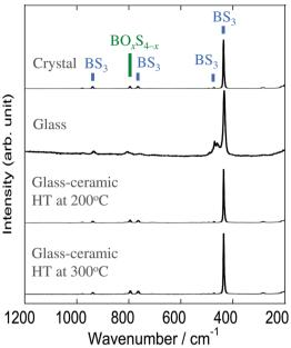
Fig. 4 Raman spectra of Na<sub>3</sub>BS<sub>3</sub> solid electrolytes
