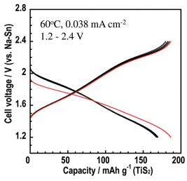
Fig. 8 Charge–discharge curves of the all-solid-state cell  $Na_{15}Sn_4/Na_3BS_3$  glass/TiS $_2$  cell at 60 °C and a current density of 0.038 mA cm $^{-2}$  in the potential range of 1.2–2.4 V.
