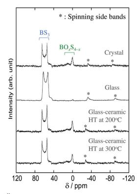
Fig. 3 <sup>11</sup>B MAS-NMR spectra of Na<sub>3</sub>BS<sub>3</sub> solid electrolytes.
