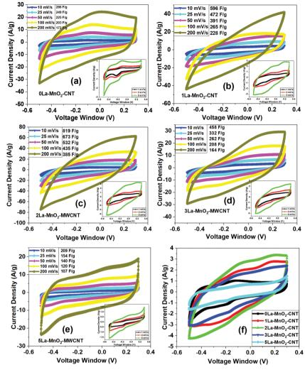
Fig. 7 CV curves of  $0La-MnO_2-CNT$  (a) and various La doped  $MnO_2-CNT$  hybrids (b-e) at varying scan rates; (insets of (a-e) show the curves at low scan rates); (f) comparative CV curves of all the samples at 5 mV s<sup>-1</sup> scan rate.
