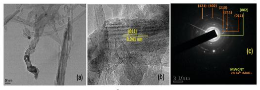
Fig. 6 (a) TEM image; (b) HRTEM image showing a single 2 mol% La $^{3+}$ :MnO $_2$  attached to CNT; and (c) SAED pattern of 2La-MnO $_2$ -CNT.
