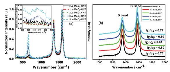
Fig. 2 Raman spectra of undoped and La-doped MnO<sub>2</sub>-CNT (a); Raman spectra showing the D band and G band of undoped and La-doped MnO<sub>2</sub>-CNT (b).
