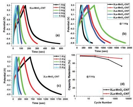
Fig. 9 GCD profiles of  $0La-MnO_2-CNT$  at different constant current densities (a); comparative GCD profiles of undoped and  $La^{3+}$   $MnO_2-CNT$  nanohybrids at 1 A  $g^{-1}$  (b); GCD profiles of  $2La-MnO_2-CNT$  at 1 A  $g^{-1}$  (c); cycle stability of  $0La-MnO_2-CNT$  and  $2La-MnO_2-CNT$  at 5 A  $g^{-1}$  up to 5000 cycles (d).
