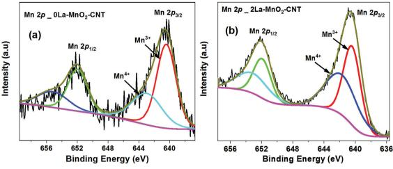
Fig. 3 XPS spectra of Mn 2p of OLa-MnO<sub>2</sub>-CNT (a) and 2La-MnO<sub>2</sub>-CNT (b).
