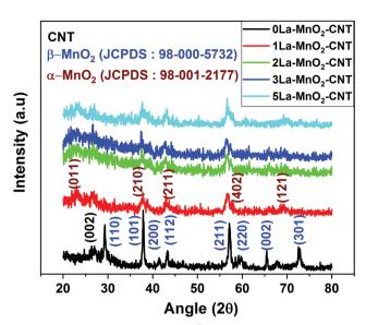
Fig. 1 XRD pattern of undoped and La<sup>3+</sup>:MnO<sub>2</sub>-CNT nanohybrid.
