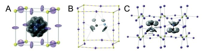
Fig. 5 Depictions of MA<sup>+</sup> cation orientations in the (A) cubic phase with ADP ellipsoids at 50% probability, (B) one orientation of the tetragonal phase with ADP ellipsoids at 50% probability, and (C) orthorhombic phase with ADP ellipsoids at 90% probability of MAPbI<sub>3</sub>, as determined by powder neutron diffraction experiments. Adapted with permission from ref. 43. Copyright 2015, Royal Society of Chemistry.
