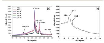
Fig. 10 Representative XRD patterns of (a) neat PCL and its biocomposites with bamboo-root flour and (b) the biofiller bamboo-root flour.
