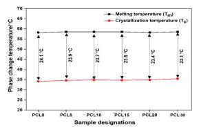
Fig. 9 The phase change temperatures ( $T_{\rm m}$  and  $T_{\rm c}$ ) and the degree of supercooling of neat PCL (PCL0) and its biocomposites with bamboo-root flour.
