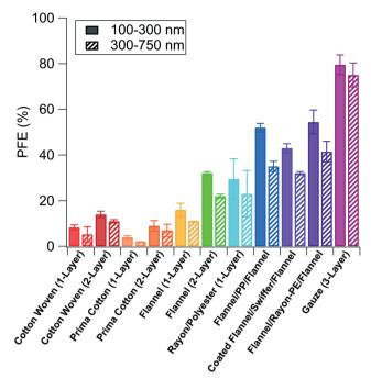
Fig. 4 Comparison of PFE for 100-300 nm and 300-750 nm aerosol size bins for selected materials of single and multiple layers, as well as in combination with multiple types of materials.
