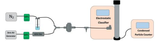
Fig. 2 Schematic of the aerosol generation setup along with the SMPS detector system.
