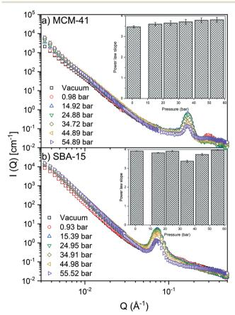
Fig. 2 The small-angle neutron scattering intensities of CO<sub>2</sub>-loaded (a) MCM-41 and (b) SBA-15 pores as a function of the wavevector and the applied pressure are shown. The insets represent the power law slope values as a function of the applied pressure.
