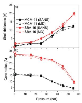
Fig. 7 The thickness of the adsorbed CO<sub>2</sub> layer determined from the small-angle neutron scattering measurements and molecular dynamics simulations (a) and the corresponding core radius (b) as a function of the applied pressure are shown. The error bars of the SANS and MD data represent standard deviations based on fittings and simulations performed in triplicates.
