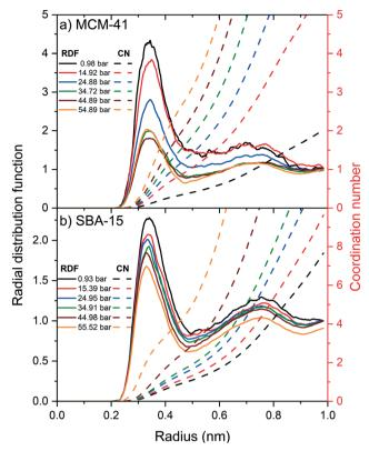
Fig. 8 The radial distribution functions and the corresponding coordination numbers of -OH-C<sub>CO<sub>3</sub></sub> in the MCM-41 (a) and SBA-15 (b) as a function of the applied pressure are shown. The simulation data are averaged over the last 10 ns of the simulation time.
