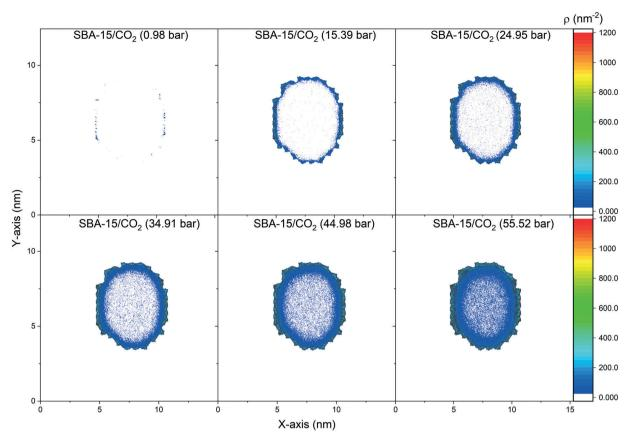
Fig. 6 The 2D density maps of the CO<sub>2</sub> molecules adsorbed on the pore walls of SBA-15 as a function of the pressure obtained from the classical molecular dynamics simulations are shown. The pore diameter of SBA-15 is 6.8 nm. The density maps are averaged over the last 10 ns of the simulation time.
