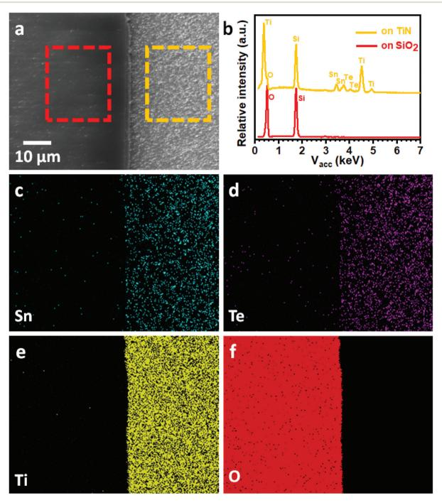
Fig. 5 (a) Top-view SEM image of a TiN/SiO<sub>2</sub> patterned substrate with SnTe selectively deposited on the TiN surface (right). (b) EDX spectra taken from the rectangular areas indicated in (a). EDX element mapping of (c) Sn, (d) Te, (e) Ti and (f) O.
