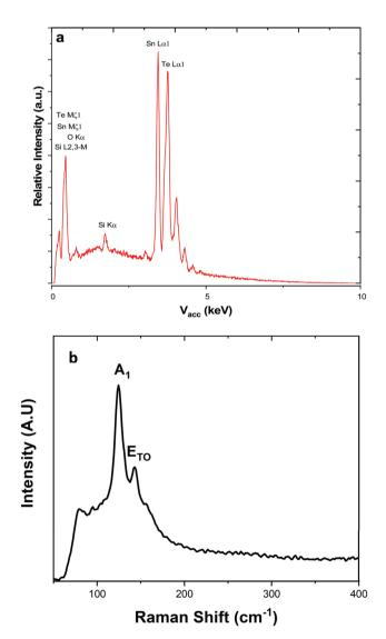
Fig. 3 (a) EDX spectrum highlighting the elements present within the SnTe film, the silicon present is attributed to the substrate. (b) Raman spectrum with the data highlighting the  $A_1$  and E modes at 124 and 143 cm<sup>-1</sup>, respectively.<sup>1</sup>
