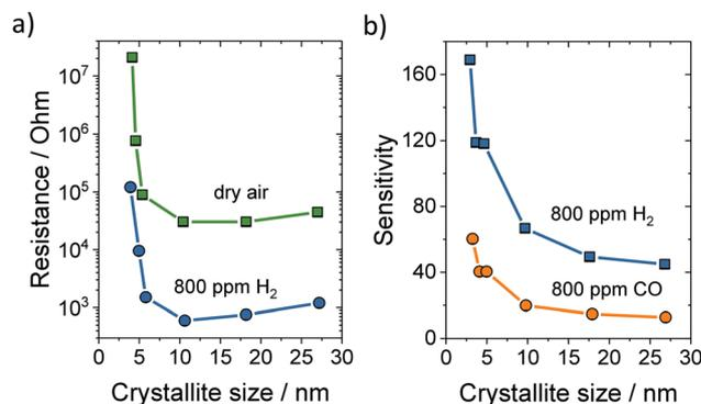
Fig. 25 (a) Electrical resistance at 300 °C in dry air or 800 ppm  $H_2$  versus the crystallite size of  $SnO_2$ . (b) Sensitivity to 800 ppm  $H_2$  or CO versus the crystallite size of  $SnO_2$ . Adapted from ref. 263 with permission.
