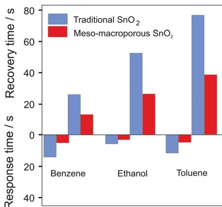
Fig. 26 Comparison of recovery and response times to 100 ppm benzene, ethanol or toluene for “traditional”  $\text{SnO}_2$  and mesoporous-macroporous  $\text{SnO}_2$ . Adapted from ref. 268 with permission.
