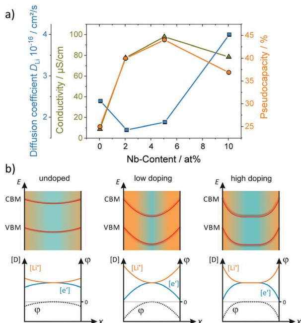
Fig. 16 (a) Electrical conductivity and pseudocapacitive charge storage of mesoporous TiO<sub>2</sub> versus the Nb doping level. (b) Schematic illustration of the surface band bending and the corresponding defect concentration for different doping situations. Adapted from ref. 156 with permission.
