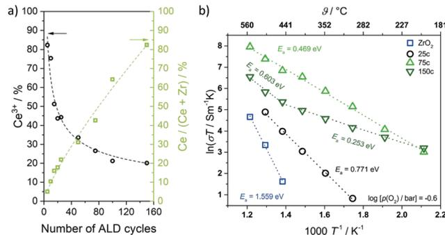
Fig. 30 (a) Ce<sup>3+</sup> content of ceria deposited onto mesoporous ZrO<sub>2</sub> thin films as function of the ALD cycle number. The Ce<sup>3+</sup> content decreases with increasing coating thickness. (b) Temperature-dependence of total conductivity for mesoporous ZrO<sub>2</sub> and CeO<sub>2</sub>-ZrO<sub>2</sub> composite thin films (25, 75 and 150 ALD cycles). Adapted from ref. 318 with permission.
