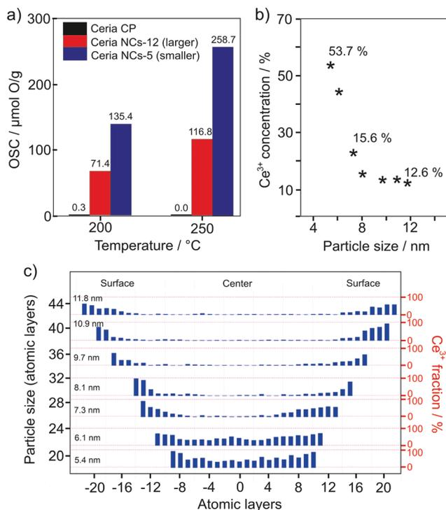
Fig. 18 (a) Comparison of the oxygen-storage capacity of  $\text{CeO}_2$  nanoparticles of different size and commercially available nanopowder. (b)  $\text{Ce}^{3+}$  content as function of the particle size and (c) valence-state distribution. Adapted from ref. 226 with permission.
