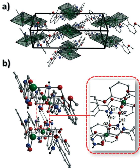
**Fig. 3** (a) Packing in **1** highlighting the individual 1-D chains stacking along the *ac* unit cell direction. (b) Two individual  $\{\text{Cu(II)}(\text{L}_3\text{H}_2)_2\}$  chains connected through inter-chain complementary hydrogen bonding represented as dashed lines ( $\text{N1(H2)}\cdots\text{O2}' = 2.03 \text{ \AA}$ ).
