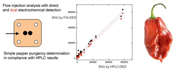
Fig. 1 (A) Schematic image of flow injection analysis with amperometric dual electrode detection using a thin layer cell with glassy carbon working electrodes. The correlation of SHU determined by HPLC-DED and by FIA-DED using E1 (upstream electrode,  $E_{DET} = 1.0 \text{ V}$ ; squares) and E2 (downstream electrode,  $E_{DET} = 0.0 \text{ V}$ ; circles) for electrochemical detection is also shown.<sup>39</sup> Reproduced with permission from ref. 39. Copyright Elsevier 2018
