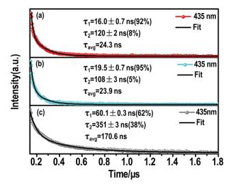
Fig. 4 Nanosecond time-resolve emission (ns-TE) decays and fittings of the (a)  $(S-\beta-MPEA)_2PbBr_4$ , (b)  $(R-\beta-MPEA)_2PbBr_4$ , and (c) ((rac)-MPEA)<sub>2</sub>PbBr<sub>4</sub> emission at 435 nm.
