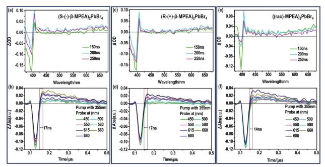
Fig. 3 ns-TA spectra of (a) (S-β-MPEA)<sub>2</sub>PbBr<sub>4</sub>, (c) (R-β-MPEA)<sub>2</sub>PbBr<sub>4</sub>, (e) ((rac)-MPEA)<sub>2</sub>PbBr<sub>4</sub> films upon excitation at 355 nm. TA onsets of (b)  $(S-\beta-MPEA)_2PbBr_4$  (d)  $(R-\beta-MPEA)_2PbBr_4$ , (f)  $((rac)-MPEA)_2PbBr_4$  films probed at different wavelength.
