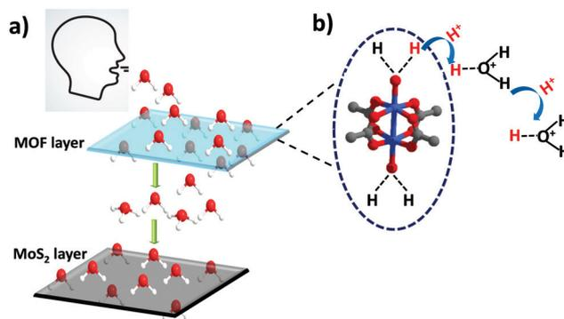
Fig. 4 Breath sensing mechanism in the HKUST-1-MoS<sub>2</sub> integrated device. (a) Adsorption and transfer of water molecules from the MOF to the MoS<sub>2</sub> layer and (b) the mechanism of proton conduction in the MOF layer involving proton transfer from acidic water molecules coordinated to the metal cluster to the solvent molecules present in the channels. Only one cluster has been shown for clarity.
