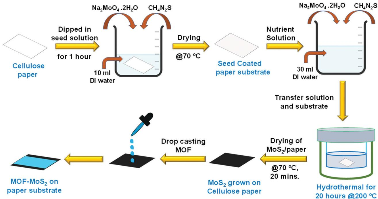
Scheme 2 Schematic illustration of growing MoS<sub>2</sub> on a cellulose paper substrate and dropcasting of MOF powder on the MoS<sub>2</sub> support for device fabrication.
