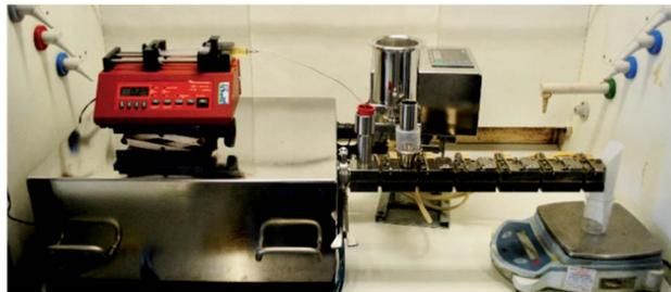
**Fig. 1** Twin screw extruder used in this study to investigate the synthesis of POCs.
