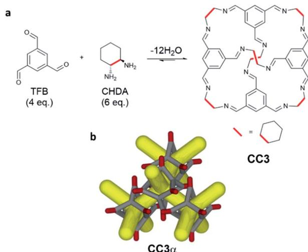
**Scheme 1** (a) Synthesis of CC3 – a [4+6] porous organic cage formed through the dynamic imine condensations of 4 equivalents of 1,3,5-triformylbenzene (TFB) with 6 equivalents of cyclohexanediamine (CHDA). Two cage enantiomers can be formed, CC3-*R* and CC3-*S*, by using the different chiralities of CHDA, (*R,R*)-CHDA and (*S,S*)-CHDA, respectively. (b) The cages can pack together window-to-window to form a 3D diamondoid pore network in the solid state (CC3 $\alpha$ ).
