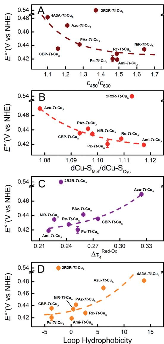
Fig. 5 Reduction potentials of the  $Tt$ - $Cu_A$  chimeras as function of (A) the experimental  $\epsilon_{450}/\epsilon_{600}$  ratio, (B) the calculated  $dCu-S_{Met}/dCu-S_{Cys}$  ratio, (C) the calculated  $\Delta\tau_4 = \tau_4$  (red) –  $\tau_4$  (ox) parameter and (D) the hydrophobicity of the ligand loop. Dashed lines are included to guide the eye. Error bars represent the standard deviation of no less than 3 independent measures.
