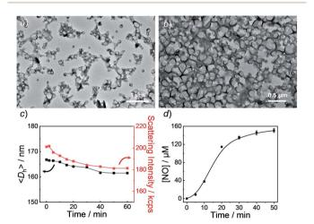
Fig. 3 TEM images of aqueous dispersions (0.1 g L<sup>-1</sup>) of BP1 vesicles (a) before and (b) after UV 365 nm irradiation. (c) Evolution of hydrodynamic diameters,  $\langle D_{\rm h} \rangle$ , and corresponding scattering intensities and (d) NO release profile of BP1 vesicles under UV 365 nm irradiation (4 mW cm<sup>-2</sup>). Data represent mean  $\pm$  s.d. (n=3).
