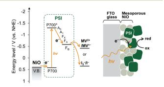
Fig. 1 Energy levels and schematic representation of the PSI-adsorbed NiO photocathode.
