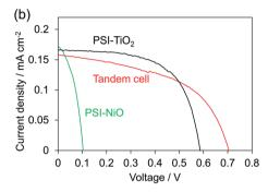
Fig. 4 (a) Schematic representation of the tandem cell power generation mechanism. (b) J-V curves under AM 1.5G (100 mW cm<sup>-2</sup>) of the tandem cell and individual n- and p-biophotovoltaic cells.
