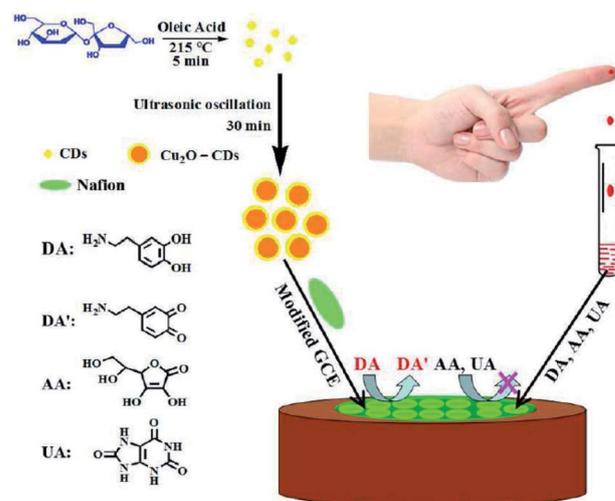
Fig. 8 A schema of the principle of electrochemical assay to detect dopamine based on cuprous the oxide-carbon dots/Nafion ( $\text{Cu}_2\text{O}$ -CDs/NF) composite film. Reprinted with permission.<sup>129</sup> Copyright 2015, RSC.
