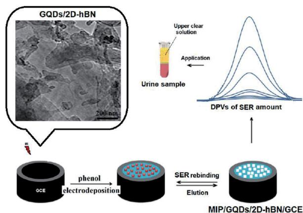
Fig. 9 MIP/GQDs/2D-hBN/GCE process. Reprinted with permission.<sup>148</sup> Copyright 2018, Elsevier.
