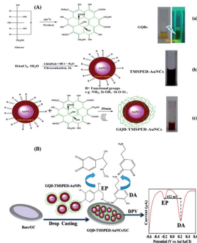
Fig. 10 A schema of the procurement process of (A) GQD-TMSPED-AuNCs nano-composites and (B) electro-chemically concurrent determination EP and DA. Reprinted with permission.<sup>153</sup> Copyright 2019, Springer.
