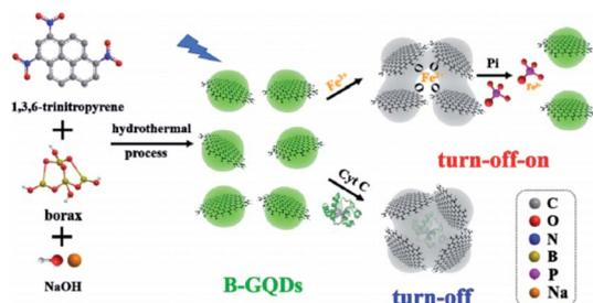
Fig. 2 A schema of the one-phase procurement of the B-GQDs to make the sensors (toward the  $\text{Fe}^{3+}$  ion and phosphate-Pi) as well as the bio-sensor (toward the cytochrome C-Cyt C). Reprinted with permission.<sup>74</sup> Copyright 2019, Elsevier.
