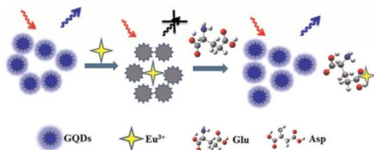
Fig. 7 The working system of the GQDs-based photo-luminescent sensors to detect Asp and Glu. Reprinted with permission.<sup>114</sup> Copyright 2015, Elsevier.
