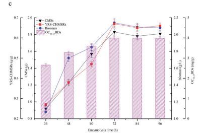
Fig. 3 The effects of the cellulase enzymatic hydrolysis on production of  $C_{14-15}BDs$ , (a) cellulase amount, (b) substrate loading and (c) enzymolysis time. All experiments were triplicated and the error bars were shown as standard deviations.
