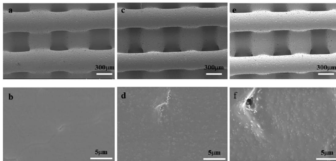
Fig. 1 SEM images: PCL scaffold at 300 μm (a), PCL scaffold at 5 μm (b), PCL/HA scaffold at 300 μm (c), PCL/HA scaffold at 5 μm (d), EPL/PCL/HA scaffold at 300 μm (e), EPL/PCL/HA scaffold at 5 μm (f).
