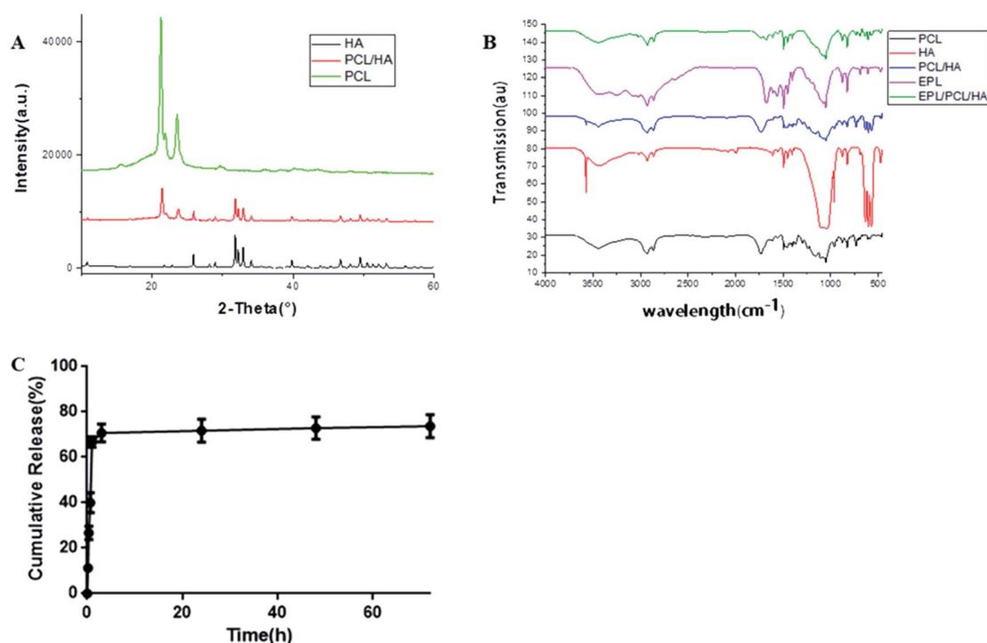
Fig. 4 (A) XRD spectra of HA, PCL and PCL/HA; (B) FT-IR analysis. (C) Release kinetics of EPL from EPL/PCL/HA scaffolds.
