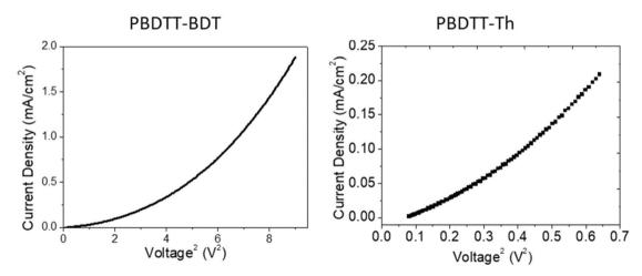
Fig. 7 J-V curve of PBDTT-BDT and PBDTT-Th measured on the probe station using SCLC model.
