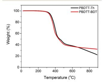
Fig. 2 TGA curves of PBDTT-Th and PBDTT-BDT.
