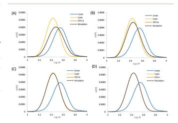
Fig. 3 Experimental SEC traces of mixtures of linear and cyclic (see Table 1). (A) PSTY-A with targeted  $w_{\rm cyclic}=49.72\%$ , (B) PSTY-B with targeted  $w_{\rm cyclic}=77.96\%$ , (C) PSTY-E with targeted  $w_{\rm cyclic}=95.68\%$ , and (D) PSTY-I with targeted  $w_{\rm cyclic}=99.50\%$ . The dashed lines are the fit using the ss to determine  $w_{\rm cyclic}$  calculated from fitting the experimental linear and cyclic distributions to the experimental distribution.
