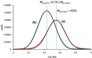
Fig. 1 SEC chromatograms of the cyclization of linear PSTY<sub>35</sub>. (A) before, and (B) after CuAAC coupling reaction. Dashed lines represent the fit using the LND method using for linear  $M_{\rm n}$  = 3674 and D = 1.068. The cyclic polymer was fit using  $M_{p,cyclic} = 0.76 M_{p,linear}$  (i.e.  $M_n = 2799$ , D = 1.068).
