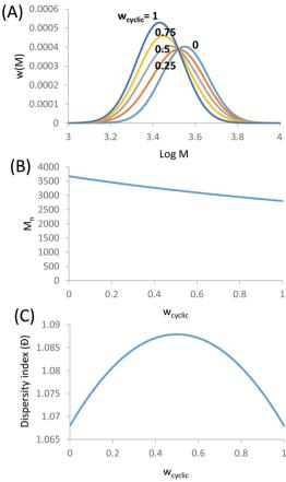
Fig. 2 Theoretical mixture of linear and cyclic distributions. (A) SEC distributions using the  $M_n$  and  $\mathcal{D}$  for linear and cyclic from Fig. 1. (B)  $M_n$  for the mixture of linear and cyclic determined from the method-ofmoments. (C) D for the mixture of linear and cyclic determined from the method-of-moments. Where  $w_{\text{cyclic}}$  is the weight fraction of cyclic to linear.
