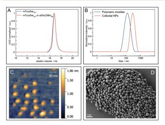
Fig. 4 HFIP GPC elugram of the block copolymer P12 (A), single-angle DLS plots of polymeric micelles and organic colloids prepared from this polymer (B), AFM image of polymeric micelles (C, scale bar 30 nm) and SEM image of organic colloids (D, scale bar  $1 \mu m$ ).
