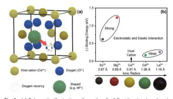
Fig. 1 (a) Schamatic illustration of a unit cell of fluorite structured ceria, showing electrosteric interaction between the acceptor dopant and charge compensating oxygen vacancy. (b) Computationally calculated binding energy (1nn) values of variously doped ceria as a function of dopant radius. The data are taken from V. Butler et al.<sup>24</sup>
