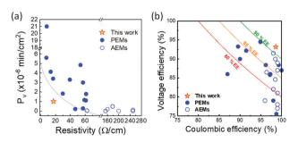
Fig. 4 (a) Trade-off between vanadium diffusivity and resistivity. (b) VRFB performance relationship among CE, VE, and EE at 40-60 mA cm<sup>-2</sup> Detailed information on the trade-off curves is available in Tables S3 and S4 (ESI†).
