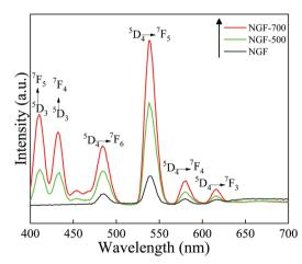
**Fig. 7** The photoluminescence emission spectra of the pristine NaGdF<sub>4</sub>:3% Tb<sup>3+</sup> phosphor crystals and NaGdF<sub>4</sub>:3% Tb<sup>3+</sup> phosphor annealed at 500 °C and 700 °C, monitored at  $\lambda_{\rm ex}$  = 228 nm. The emission intensity increased at higher annealing temperatures.
