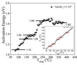
**Fig. 12** Activation energy (eV) vs.  $T_{\text{stop}}$  (°C) plot resulting from the IR method after the  $T_{\text{m}}$ – $T_{\text{stop}}$  procedure for the NaGdF<sub>4</sub>:3% Tb<sup>3+</sup> phosphor irradiated with gamma radiation of 10 kGy doses. A plot of  $T_{\text{m}}$  as a function of  $T_{\text{stop}}$  for the NaGdF<sub>4</sub>:3% Tb<sup>3+</sup> phosphor as an inset image.
