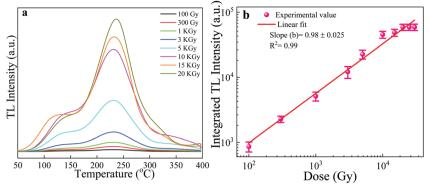
Fig. 9 TL glow curves of the NaGdF<sub>4</sub>:3% Tb<sup>3+</sup> phosphor irradiated with various doses (100 Gy to 20 kGy) of gamma rays from a <sup>60</sup>Co source (a). Linear TL response of the NaGdF<sub>4</sub>:3% Tb<sup>3+</sup> phosphor as a function of irradiation dose (b).
