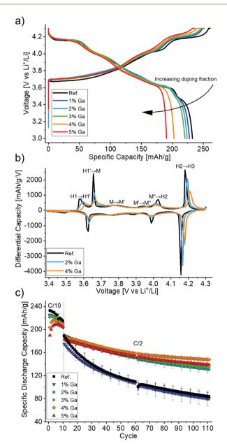
Fig. 5 Electrochemical data for undoped and Ga-doped LNO from galvanostatic cycling of half-cells at 25  $^{\circ}$ C in the voltage range between 3.0 and 4.3 V vs. Li<sup>+</sup>/Li. (a) 1st cycle voltage profiles. (b) 3rd cycle differential capacity plots. Only selected samples are shown for clarity. (c) Specific discharge capacity over 110 cycles.
