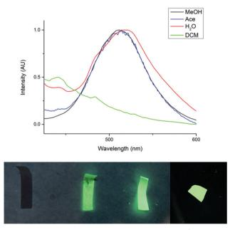
Fig. 4 (top) Solid-state photoluminescent emission spectra<sup>a</sup> and (bottom) digital photographs of F1 treated with different solvents<sup>b.c</sup>.  $^{a}\lambda_{ex}=368$  nm (excitation wavelength).  $^{b}$ Papers exposed to UV irradiation ( $\lambda=365$  nm).  $^{c}$ (from left to right) dichloromethane, acetone, methanol, water.
