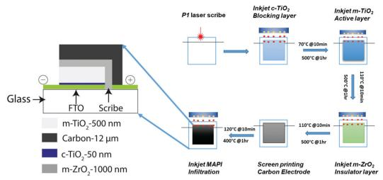
Fig. 1 Device architecture of the MPSC with desired layer thicknesses in cross section view. Process flow demonstrating inkjet printing of four layers consisting of compact titania (c-TiO<sub>2</sub>), mesoporous titania (m-TiO<sub>2</sub>), mesoporous zirconia (m-ZrO<sub>2</sub>) and infiltration of methyl ammonium lead tri-iodide (MAPI) perovskite precursor. Yellow dots represent the print head nozzles while red dots represent the ejected droplets
