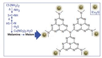
Scheme 1 The formation mechanism of embedded copper sulfide in the carbon nitride matrix
