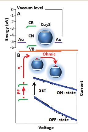
Fig. 5 (A) The energy diagram of the Au||CSCN||Au device. (B) The electron transport mechanism within the device. The electron transfer, from the HOMO to the LUMO of the CN system, followed Poole-Frenkel emission for the OFF-state and the ohmic mechanism was followed for the ON-state through the Cu<sub>2</sub>S particles
