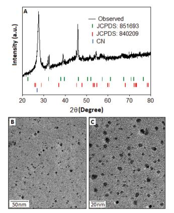
Fig. 1 (A) X-ray diffraction pattern of  $Cu_{2-x}S$  particles embedded within the carbon nitride matrix. The pattern consists of mixed phases of Cu<sub>1.8</sub>S (green bar, JCPDS: 851693) and Cu<sub>2</sub>S (red bar, JCPDS: 840209) compositions. The hexagonal phase of carbon nitride (blue bar) is identified in the diffraction pattern. (B and C) TEM images of copper sulfide nanoparticles on the carbon nitride matrix, with different magnification.
