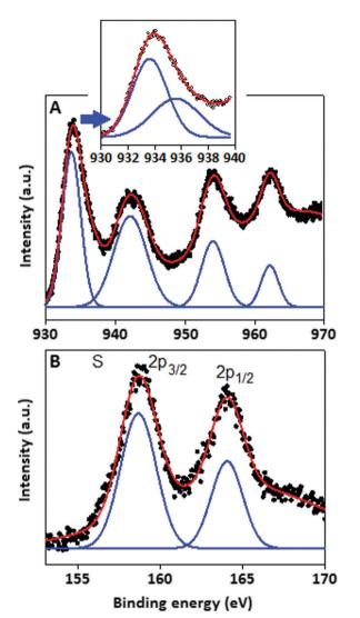
Fig. 2 X-ray photoelectron spectroscopy characteristics of the copper sulfide particles. XPS signal for (A) copper species and (B) sulphur species.
