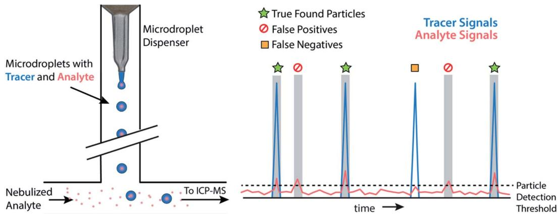
**Fig. 3** Schematic diagram of a generic tracer-analyte experiment with microdroplets. Low-abundance “analyte” species in the microdroplets are treated as analyte particles and measured *via* sp-ICP-TOFMS. The accuracy of analyte particle detection is assessed based on the presence or absence of tracer signal concurrent with the found analyte particle signals.
