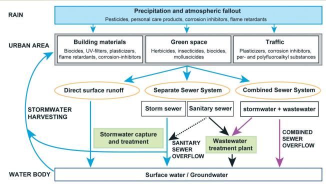
Fig. 1 Sources of hydrophilic trace organic contaminants (hyphil-TrOCs) in urban stormwater and input paths of stormwater- and wastewaterderived hyphil-TrOCs into receiving waters. Stormwater harvesting for the urban water supply requires stormwater capture and treatment
